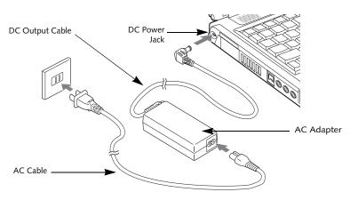
Figure 3-1 Connecting the AC Adapter
